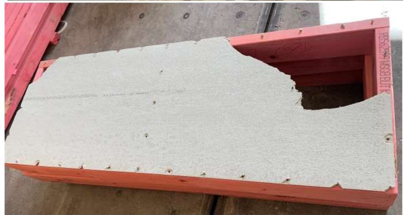
Figure 4. Typical specimen mode showing fixing pull-throughs and sheet fractures.
