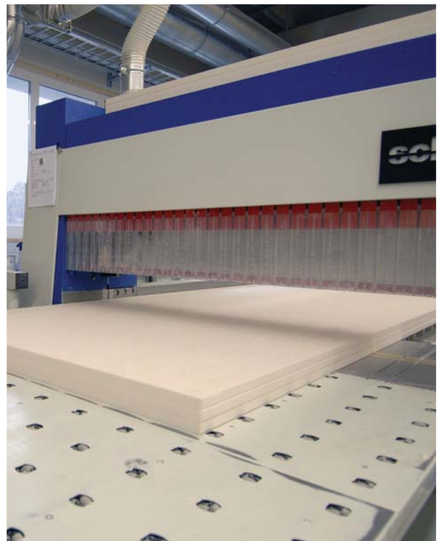
Cutting Promat boards with "Schelling 1" cut-to-size machine
